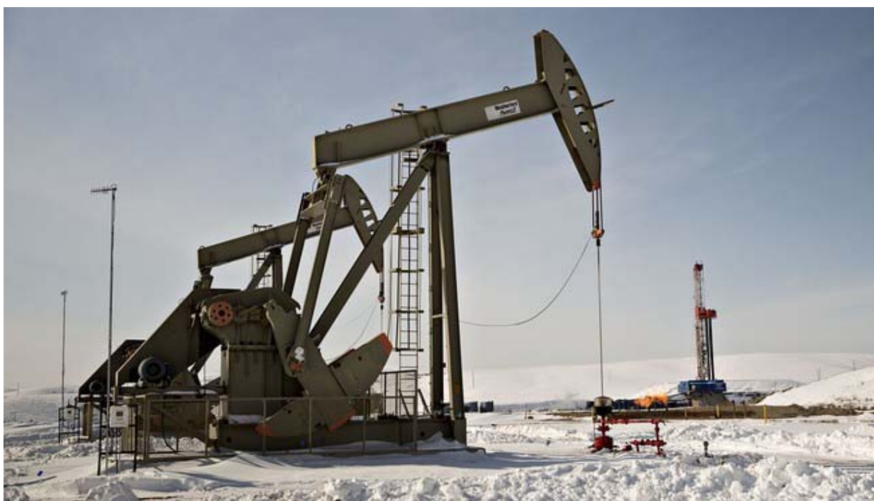
A pumpjack operates as a drill rig sits on a well pad in the Bakken Formation in Williston, North Dakota.
